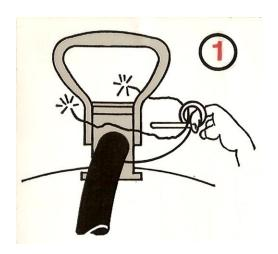
Pull the ring pin while breaking the plastic safety strap
